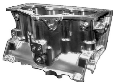
Figure 2. External View of the Five-Stroke Engine Block
